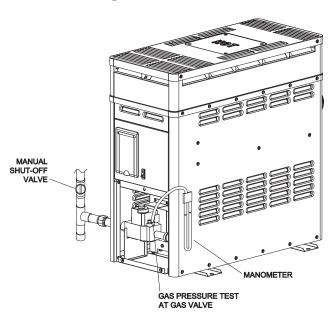
Fig. 9: Location of Gas Pressure Adjustment
