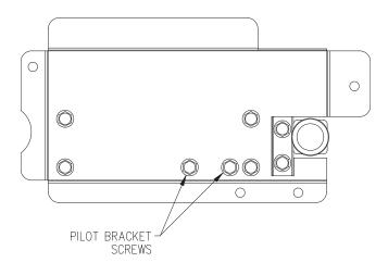
Fig. 29: Pilot Bracket Screws
