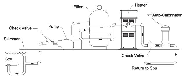
Fig. 1: Spa/Chlorinator Setup
