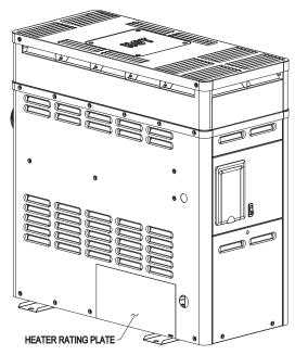
Fig. 2: Location of Heater Rating Plate
