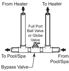
Fig. 13: Auxiliary Bypass Valve
