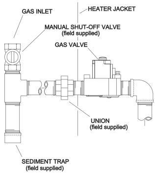
Fig. 7: Gas Line Sediment Trap
