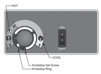
Fig. 17: Water Temperature Thermostat
