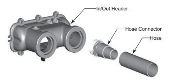
Fig. 11: Optional In/Out Header for 1-1/2" (3.8 cm) or 1-1/4" (3.2 cm) Hose Connection
