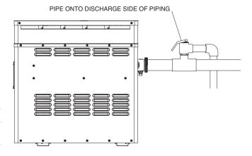
Fig. 14: Pressure Relief Valve Installed
