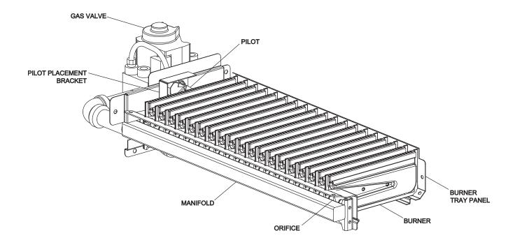
Fig. 26: Burner Tray Assembly
