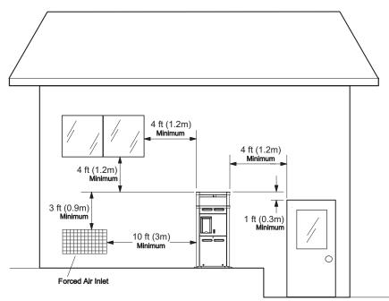
Fig. 5: Outdoor Installation Clearances
