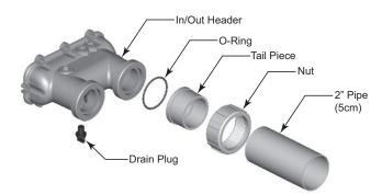
Fig. 10: In/Out Header for 2" Installation
