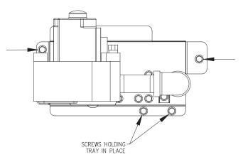
Fig. 27: Gas Valve Removal
