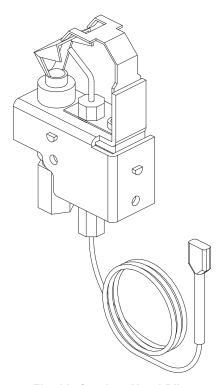
Fig. 28: Spark to Hood Pilot
