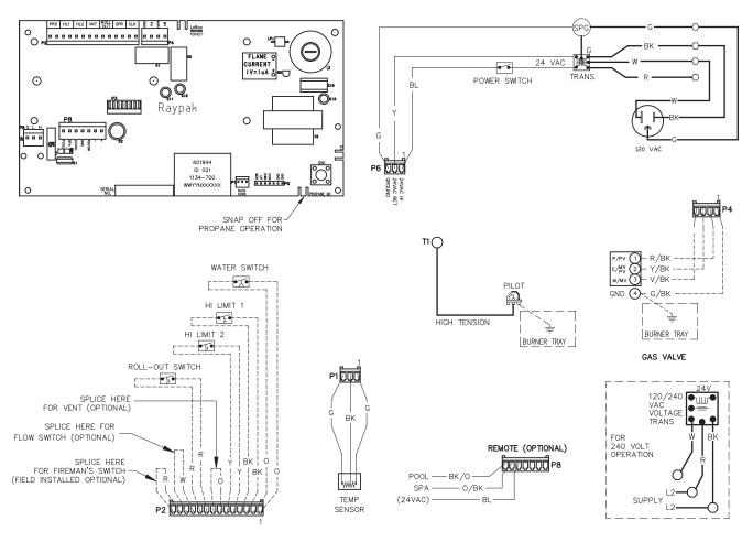
Fig. 20: Wiring Diagram—Digital Models
