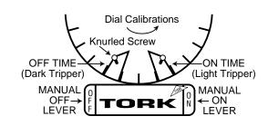
**TO SET DIAL TO TIME:** Turn dial counter-clockwise until correct time is indicated by arrow on nameplate.
