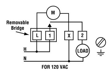
For separate motor terminals, remove bridge from terminals L & 1.
